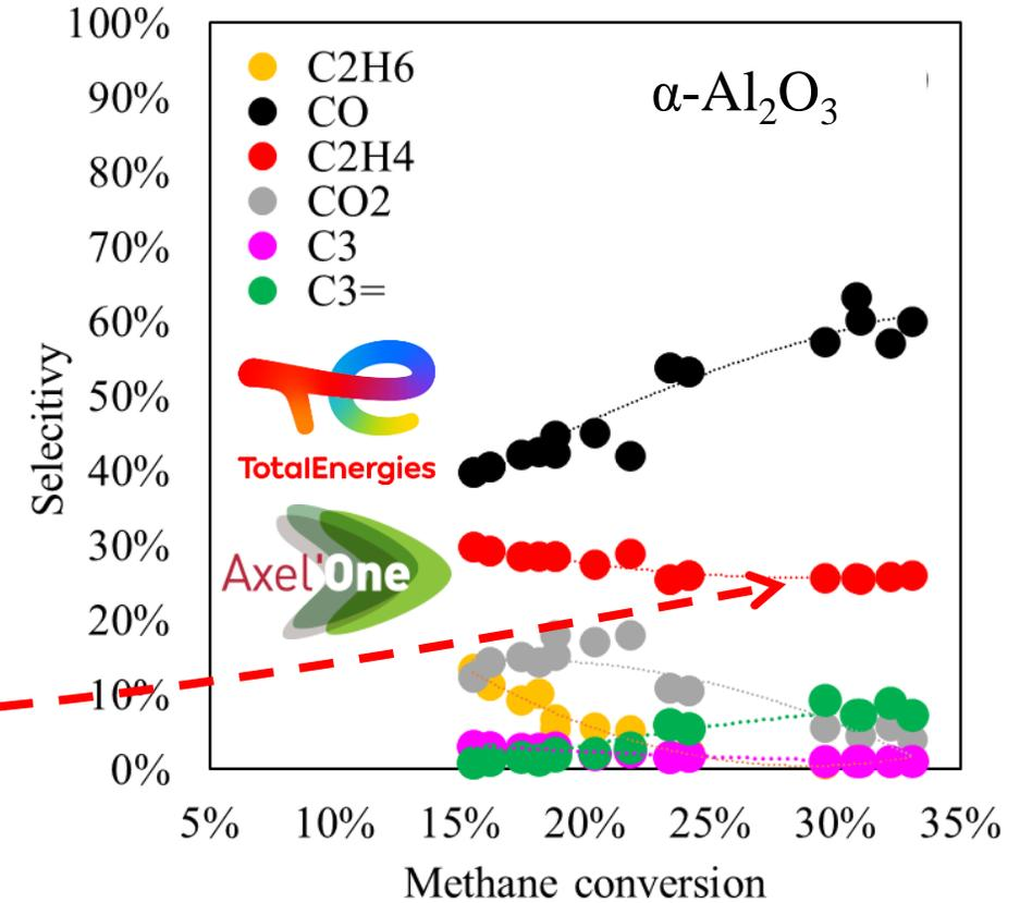
$T = 950 - 1000 \text{ }^\circ\text{C}; p_T = 1 - 3 \text{ bar};$
